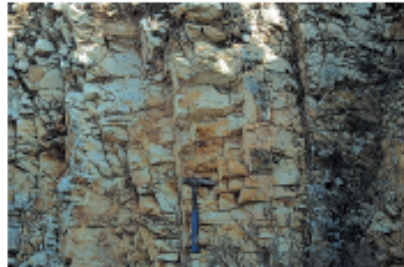
Ordovician quartzite. Fair quality. High fracturing degree. Very hard intact rock.
